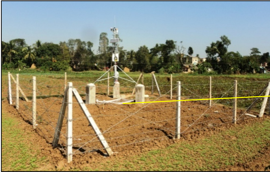
Test-bed for monitoring meteorological and soil moisture dynamic in the Jorkul Village
